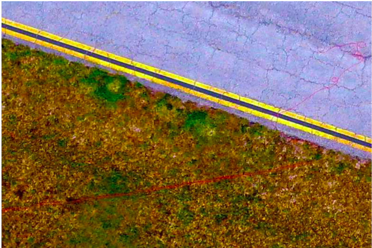
Illustration 3: In this enhanced crop of image #233, the red bungee cord used for launching the UAS is visible stretching across the grass and coiled up on the runway. The bungee cord is ½ inch in diameter.
