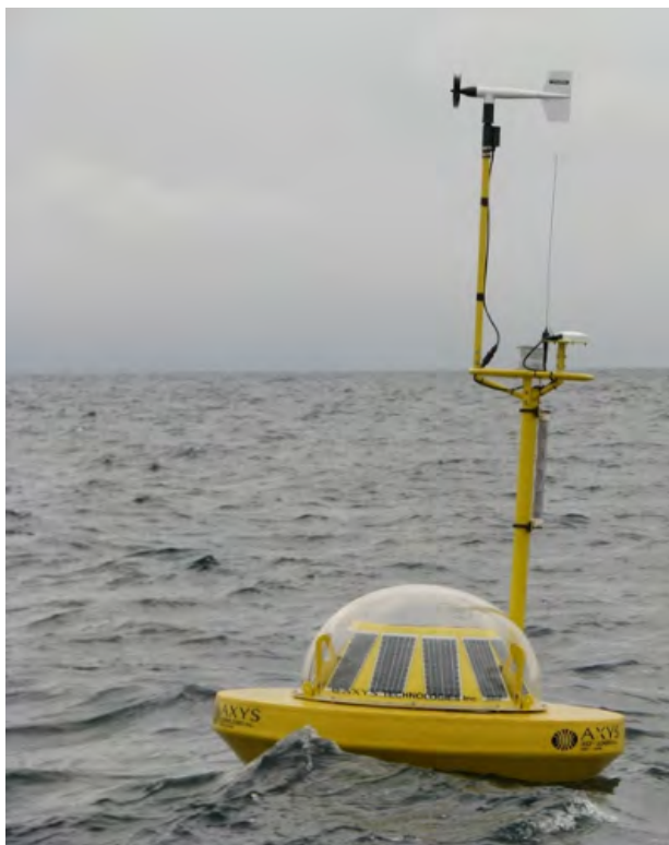
Figure 1. Axys “Watchmate” buoy. This unit measures wind, waves, and air/water temperature. The unit for the Bering Strait will be modified to include “twinned” wind sensors, a precaution against the possibility of icing.
