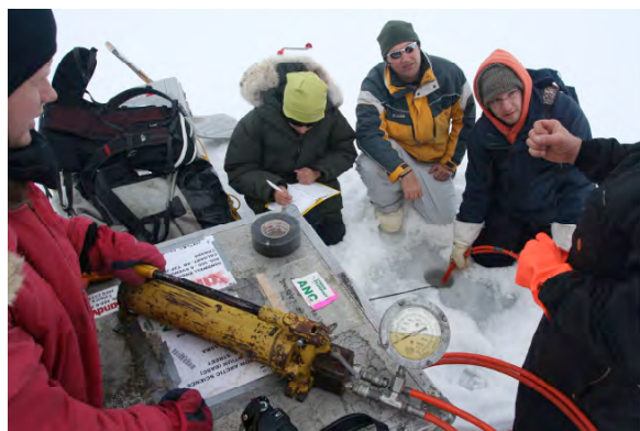
Figure 2. Students conducting measurements of ice strength with borehole jack tests.
